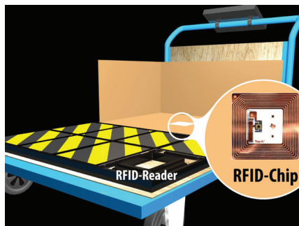
Figure 3. RFID antenna array for identifying articles and their location on the MICA trolley
